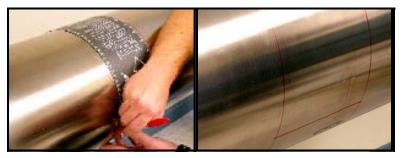
Figure 3-14: Marking the 3 o'Clock Position
